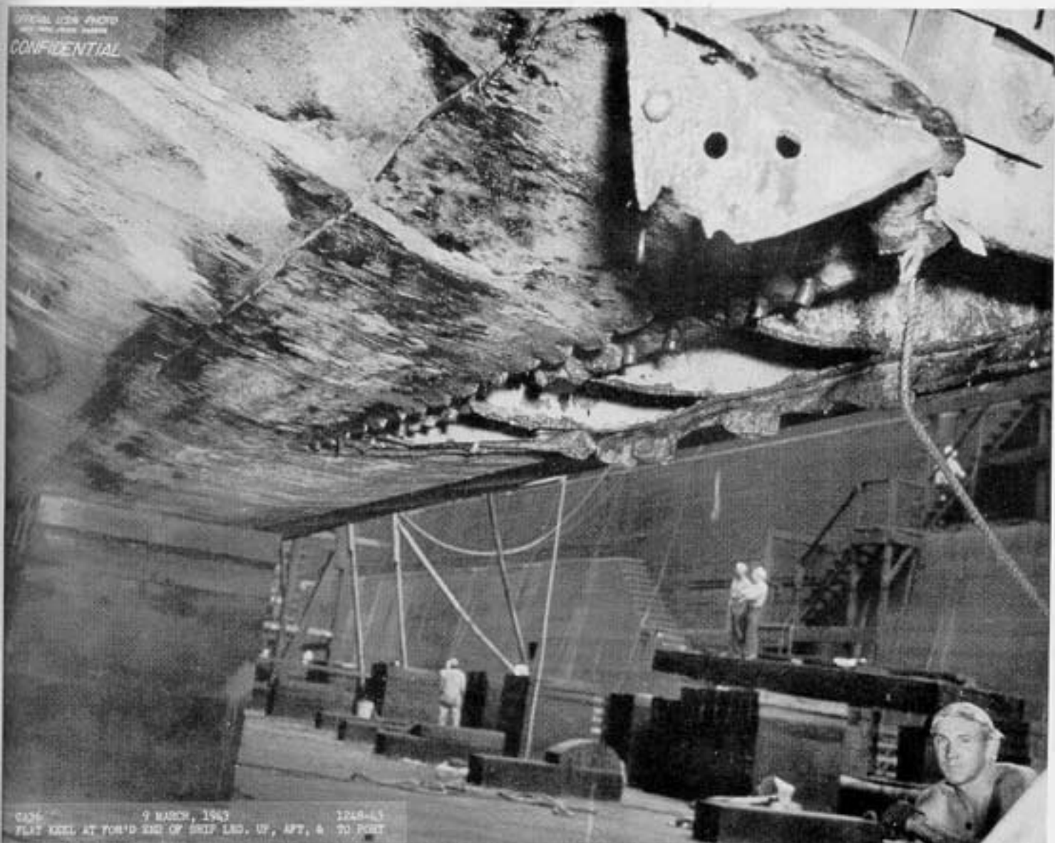
Photo No.18: USS MINNEAPOLIS - Flat keel frame 20 looking aft and to port.
