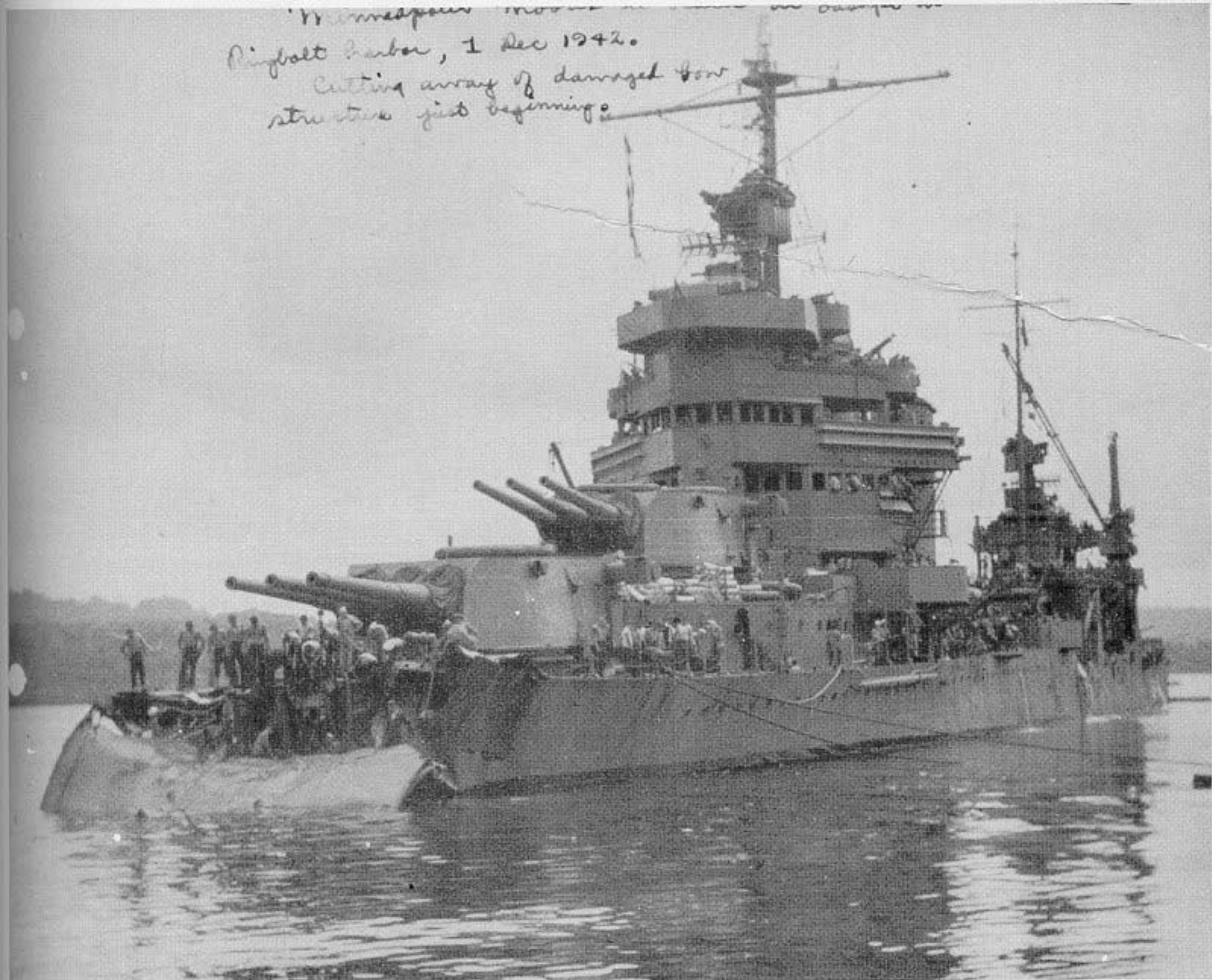
Photo No.15: USS MINNEAPOLIS - View of damaged bow before it was cut away.
