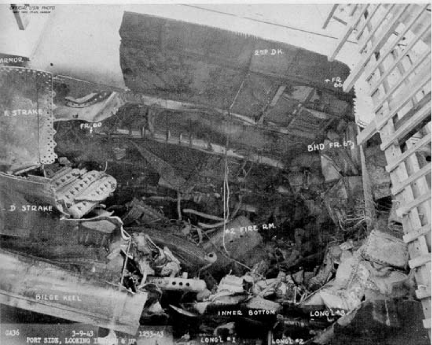
Photo No.22: USS MINNEAPOLIS - Port side looking aft No. 2 fireroom.
